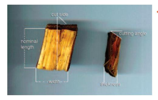
Measurement of wood chips.
